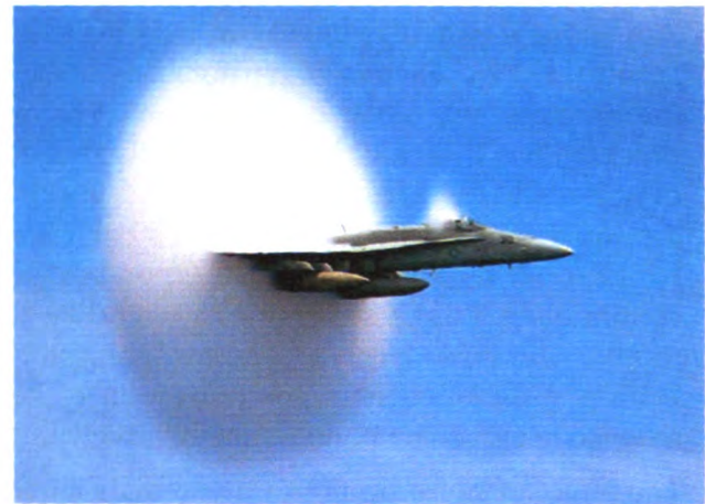
AN EXAMPLE OF A VAPOR CLOUD AROUND AN F/A-18 HORNET AT MACH 1 IN HIGH HUMIDITY CONDITIONS. (PHOTOGRAPH BY ENSIGN JOHN GAY, USS CONSTELLATION ).
